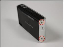
• Open the camera by removing the 5x4.0 mm external screws with the 1.0 flathead.
