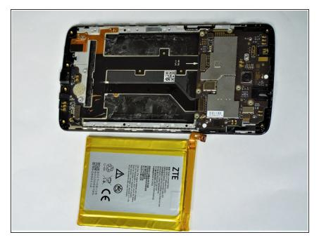
With the battery removed, you can now insert the new battery or replace other parts within your phone.
