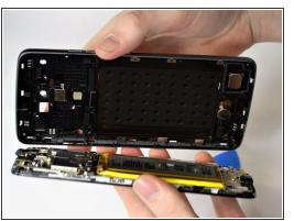
• Use a plastic opening pick between the screen and side trim battery cover to remove the screen.
