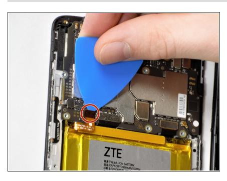
On the top left of the battery, flip the metal clips with a pick and remove the battery ribbon from the shell.
