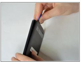
Starting at one corner, wedge the plastic opening pick underneath the plastic backing to start undoing the tabs that connect the backing to the phone. There are 3 tabs on top and bottom, and 6 on each side.
