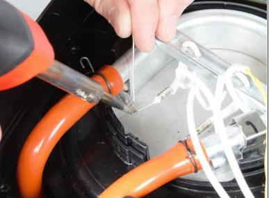
• If heating element contacts are disconnected, use soldering iron with soldering wire to re-bond the contacts.
