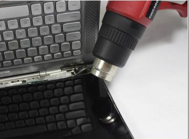
Using a heat gun, carefully apply heat evenly across the glass.
