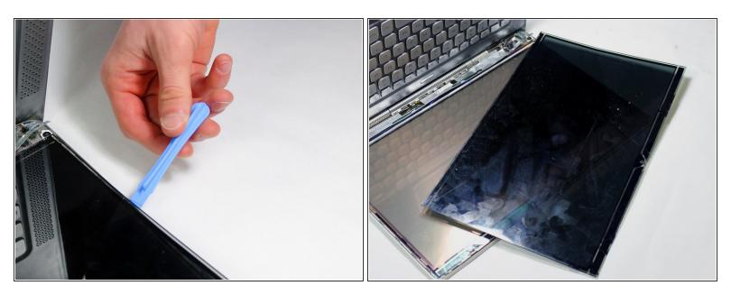
Using the iFixit opening tools, carefully pry the glass off the screen.
