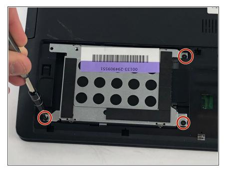
Again with the JIS 00, unscrew the three 5.7mm screws holding the hard drive in place. These can be found on small brackets on the four corners of the drive.
