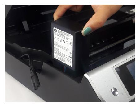
• Pull the AC adaptor up and out of its casing
