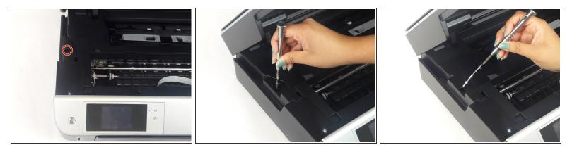
• Locate 13mm TR10 Torx Security screw behind screen and remove using Torx screwdriver.
