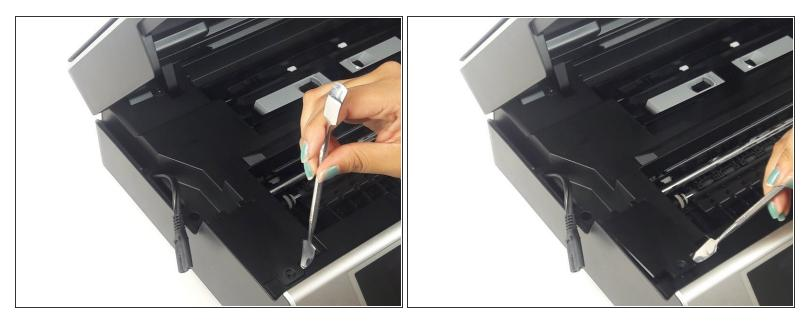
• Use a metal spudger around the edge to remove AC adapter cover.
