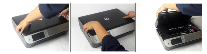
• Open the the printer by lifting the top section. Make sure you're lifting from the lowest portion of the scanner section.
