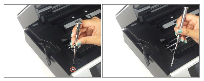
▶ Locate 13mm TR10 Torx Security screw behind screen and remove with screwdriver.
