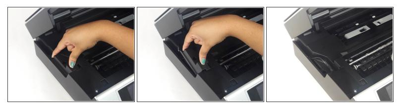
• Remove case covering by lifting it up to reveal the power cord.
