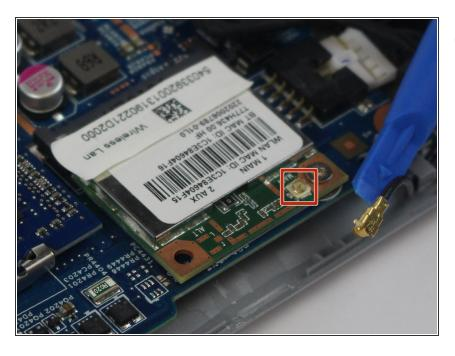
Remove the wire connector from the network card using a plastic opening tool.
