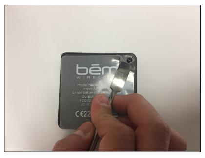
Use the metal spudger to peel back the rubber from the bottom of the auxiliary charging base to reveal the screw.
