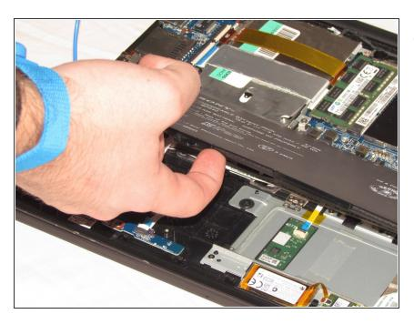
Lift the battery up and pull it out of the laptop.
