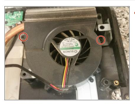
Remove the two M2.5x8 screws securing the CPU fan to the base, and remove the fan.
