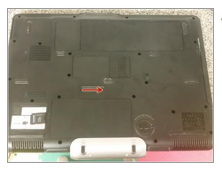
Slide battery latch to the right as pictured to release the battery.
