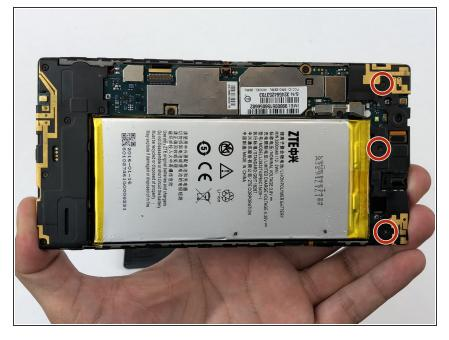
Remove the three 1.6mm Phillips #0 screws from the plastic cover on the motherboard.
