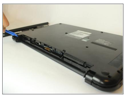
Use a plastic opening tool to lift and remove the bottom panel.
