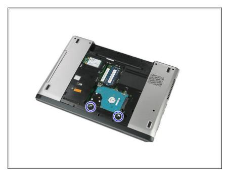
Remove the screws that secure the hard drive to the system.
