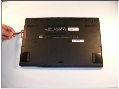
Use the spudger to slowly work your way around the perimeter starting at the marked location to pop the bottom cover off.
