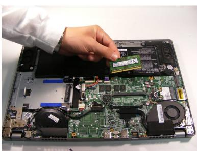
Pull back the brackets holding the RAM in place and remove the RAM.
