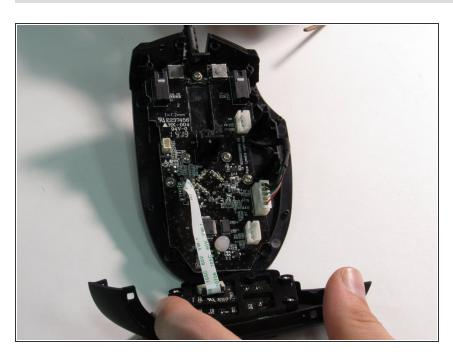
Insert the blue striped ends into the white connection port on the mainframe as well as the frame with the buttons.
