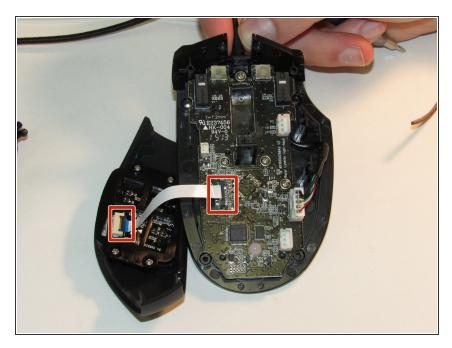
Flip back the black plastic that holds the white connection strip in place on the side panel and the main panel.
