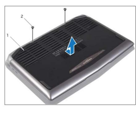
Slide the base cover toward the back of the computer and align the screws holes on the base cover with
