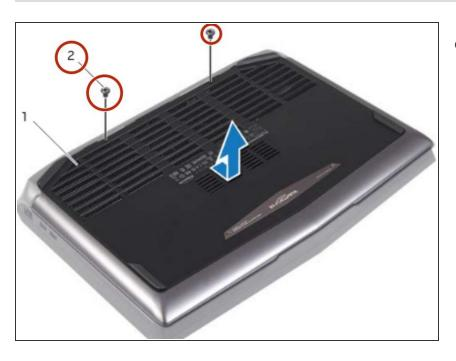
Remove the screws that secure the base cover to the computer base.
