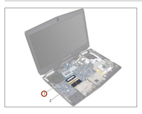
Slide the memory module into the connect or at a 45-degree angle, and press the memory module down
