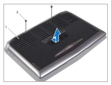
Align the tabs on the **new** base cover with the slots on the computer base
