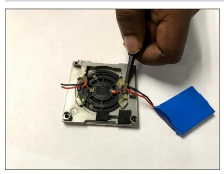
Remove the wires from the speakers battery using the tweezers or by gently removing them by lightly pinching.
