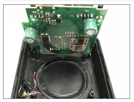
Remove bus wire from the speaker's motherboard and lift the motherboard out of the speaker.
