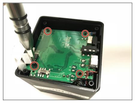
• Use the J0 screwdriver to remove all four 10mm screws from the motherboard.
