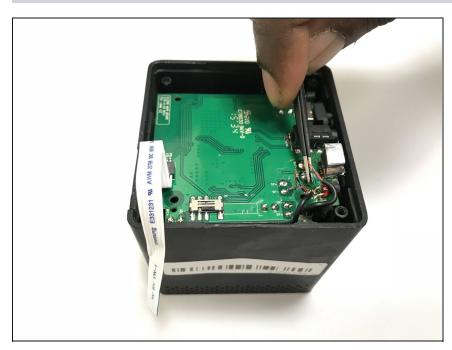
Remove the red/black wires in addition to the blue/white wires using the <u>tweezers</u>.
