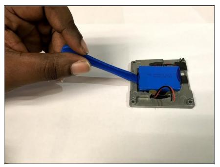
• Remove the speakers battery from its metal base, utilizing the plastic opening tool.
