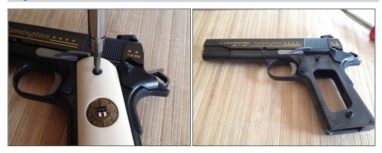
Use flathead to remove 4 screws (2 on each side) to remove the grips.
