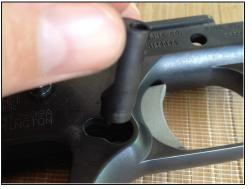
While pressing on the magazine release, use a small flathead (or the narrow angled edge of your leaf spring from the grip, it was designed with this purpose in mind) and turn the screw 90 degrees and it will pop loose for removal.
