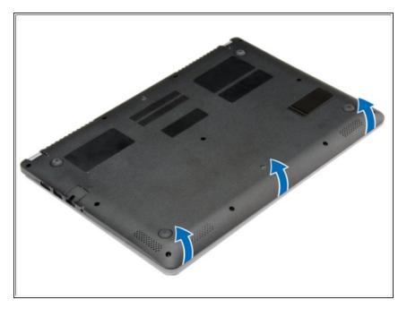
Pry the base cover along the edges to loosen it.
