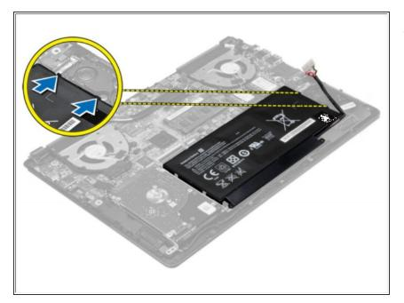
Release the tabs that secure the battery in the battery bay.
