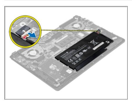
Disconnect the battery cable from its connector on the system board.
