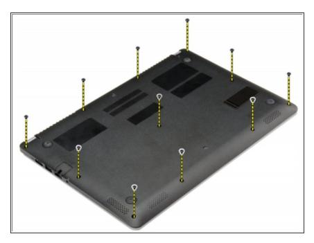
Remove the screws that secure the base cover to the computer.
