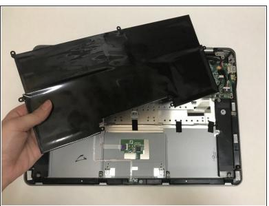
Use the plastic opening tool or your fingers to pry the battery up and pull it from the laptop.
