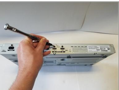
Two outer 8.1mm screws located above the HDMI ports hold the motherboard in place and must be removed. Remove these with a #1 Phillips head screwdriver.
