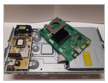
After the final screw is removed, the motherboard can be easily lifted out of the case without disturbing any of the other device components.
