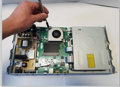
The two 6.5mm screws holding the fan in place on opposing corners must be removed with a #1 Phillips head screwdriver to change the fan.
