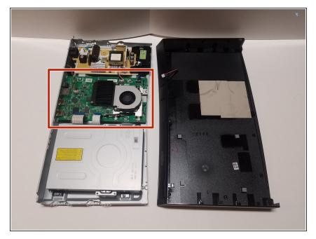
• The motherboard is in the middle of the device and has all wires and connections of the device components running to it. The fan identified as fan A is located on top of it and must be removed first.
