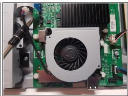
There is one wire connecting the fan to the motherboard that must be unplugged in order to release it. To unplug, use your fingers to pinch the white clip at the end and gently pull upwards to release.
