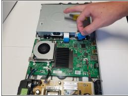
Once the fan is removed, the wires should be disconnected from the motherboard, as shown.
