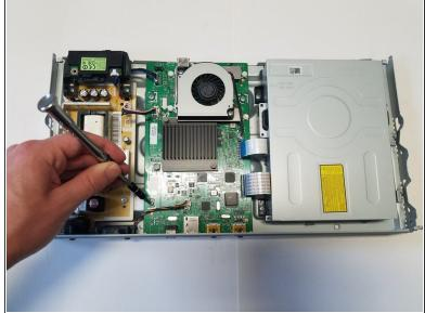
Three inner 6.5mm Phillips #1 screws hold the motherboard to the base of the frame, and must be unscrewed next.
