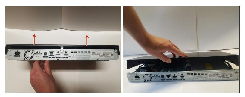
From the back, lift the case upwards away from the unit then forwards, releasing the prongs on the front.
