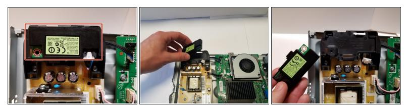
• Pull on the module from the sides and be sure not to pull on the stand that is screwed into the frame. The Wi-Fi module can then be pulled out of the clips and off the stand.
