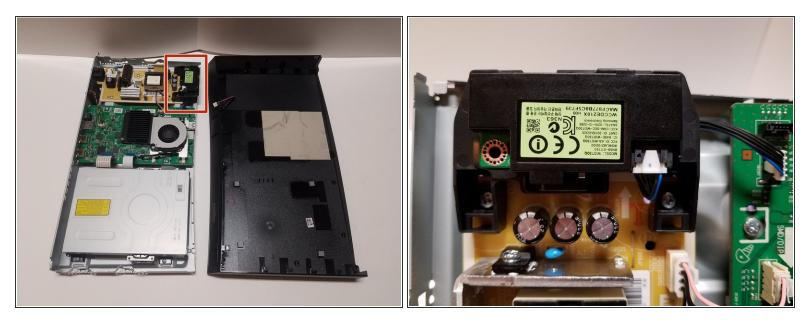
The wifi module is clipped into place in the corner of the device. There are no screws or adhesives holding it down.
