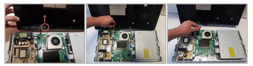
• There is one group of wires located towards the front of the case and attached directly to the motherboard and the case. Using two fingers in a pinching motion, release the wire from the clip and disconnect it.
