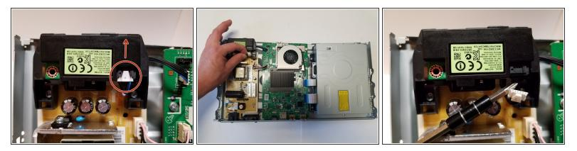
• There is one wire plugged into the Wi-Fi module that has to be removed in order to allow the range of motion to remove the module. Simply pinch the white plastic end of the wire and pull it out.
