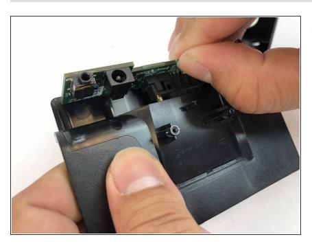
Once apart, lift the docking station motherboard up from the two pins that are located on the interior of the front casing.
