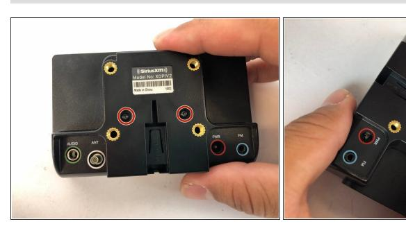
Remove the two 7.6mm Torx T6 screws from the back of the docking station.
