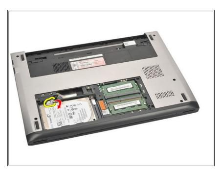
• Carefully pry up and remove the hard drive from the computer.
