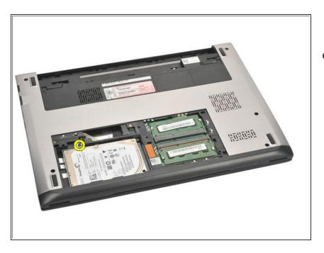
Remove the screw that secures the hard drive in place.
