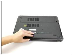
A Remove the battery to avoid electrical discharge while working with this system.
