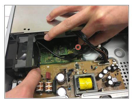
Remove the optical drive cooling fan by gripping the ribbon connector at M11 and gently remove by pulling away from the slot.
