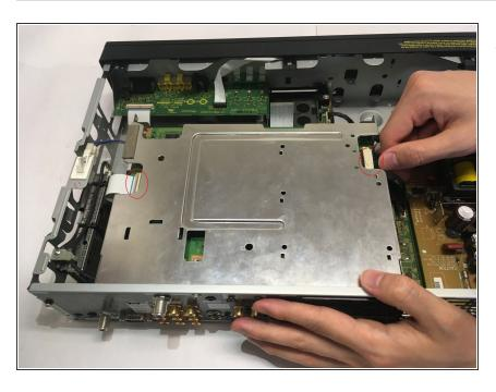
Unplug ribbon cables D4 and D5. To unplug D4, flip the gate up and pull the ribbon away.
