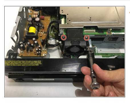
Remove the two 6.4 mm Phillips mounting screws on the optical drive cooling fan.
