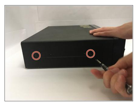
Remove the two 6.4 mm Phillips screws on each side of the device's casing.
