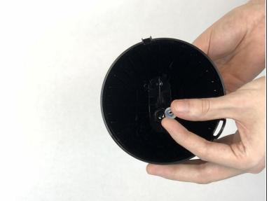
While pressing up on the drip spring mechanism, remove the clear round plastic retainer holding the mechanism in place.
