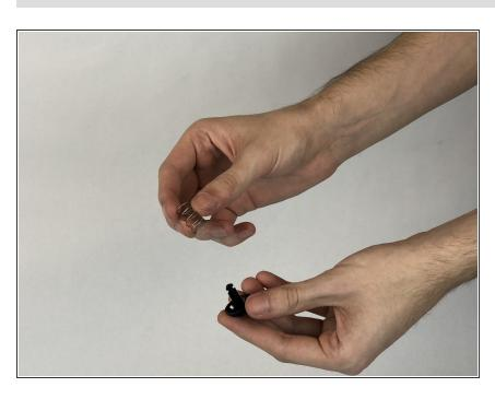
Remove the spring from the dripper.
