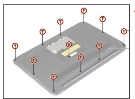
Use a Phillips screwdriver to remove the eleven screws securing the base cover.
