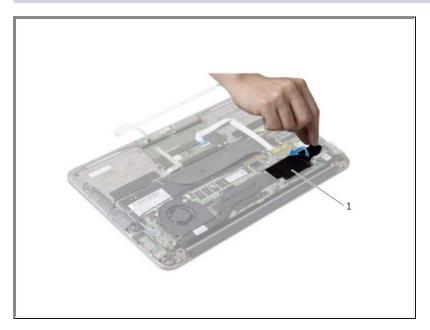
• Peel the tape that is adhered over the solid-state drive.
