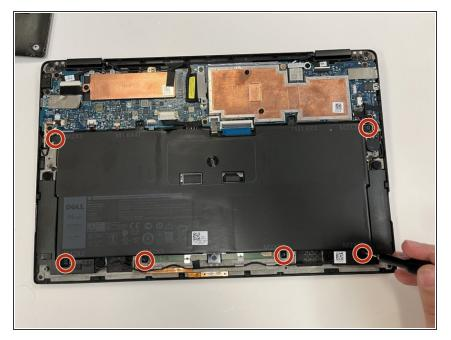
Use a Phillips #000 screwdriver to remove the six screws (M2x3) that secure the battery to the palm-rest assembly.
