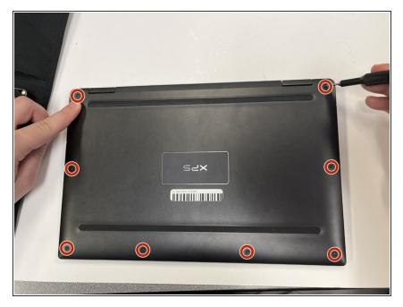
Use a Torx T4 screwdriver to remove the eight screws (M2x3) that secure the base cover to the palmrest assembly.
