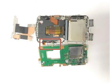
Pull the motherboard off of the main body of the camera.
