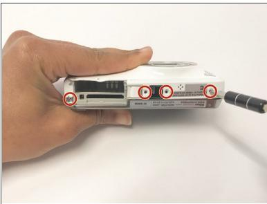
Remove all 4 screws from the bottom face of the camera using a Phillips #00 head screwdriver (found in iFixit tool kit).
