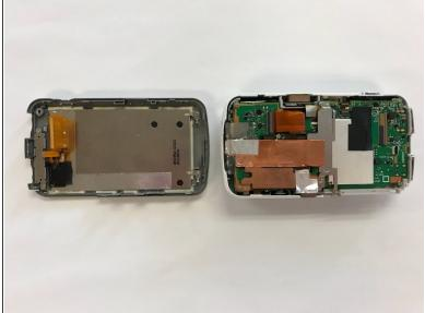
Using a plastic tool, pry open the back panel of the camera. Be careful not to apply too much force and damage the camera.
