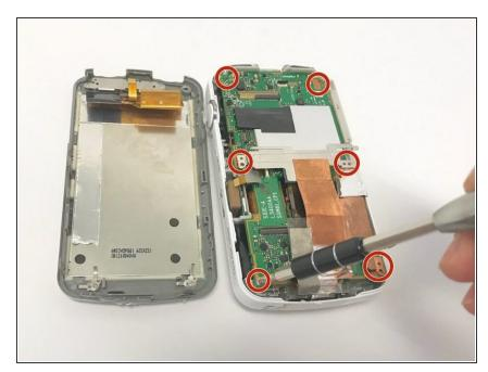
Unscrew all 6 visible screws that secure the motherboard into place using a Phillips head screwdriver (found in iFixit tool kit).
