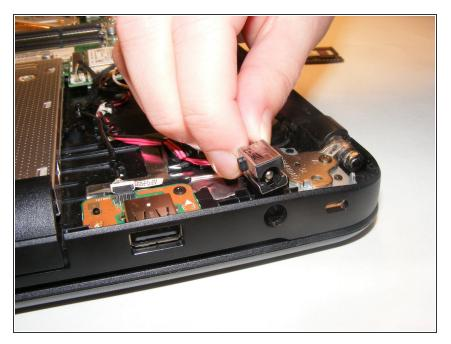
• Locate the power jack at the back, right-hand side next to the USB port.
