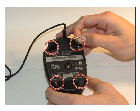
Peel back the two teflon tape from the top corners and the one larger one from the bottom with a spudger.
