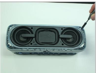
Once you have removed the outer blue casing, four T-8 screws (15 mm long) will be revealed on each corner. After removing these screws, simply pull the top part of the speaker way from the body to get the the inner part of the speaker.
