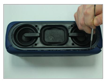
Pry the two rubber end pieces loose enough to pry off two pieces of the long plastic casing from the speaker body using a metal spudger.
