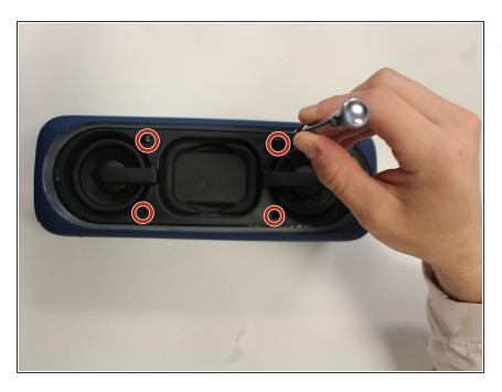
Remove the four T-8 screws (15 mm long) from the black speaker face.
