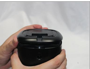
Remove the bottom cover by squeezing the protective cover slightly while pushing up with your fingers.
