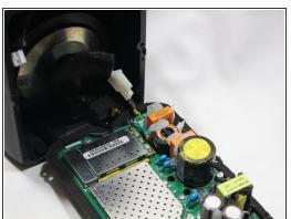
• Using the pointed end of the spudger, disconnect the red, green, and yellow cables connecting the WiFi transmitter/receiver.
