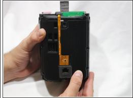
• Remove the six 9mm Torx T8 screws from the motherboard panel.
