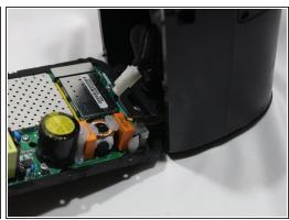
Disconnect the power adapter plug from the motherboard using your thumb.
