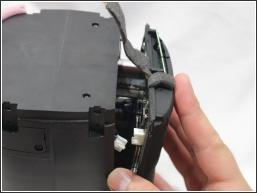
• Using your thumb, disconnect the speaker cable from the motherboard.
