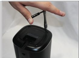
Remove the four 10mm Torx T10 screws from the bottom of the speaker.
