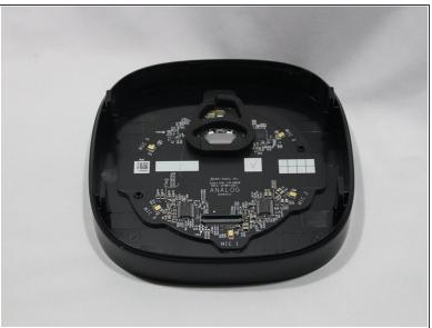
Pull the control panel away from the speaker to separate.
