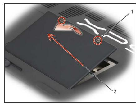
Turn the computer over, loosen the captive screws on the memory module cover, and then remove the cover.
