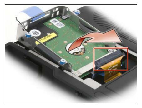
Carefully remove the SATA cables from the hard drive or drives that are installed in the cage.
