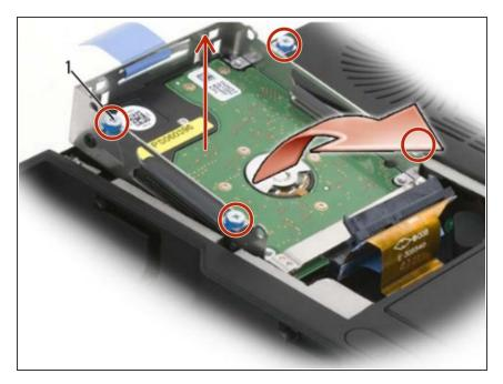
Loosen the four captive screws on the hard drive cage and then lift the pull-tab to flip the cage towards the center of the computer so that the SATA cables and connec tors are accessible.
