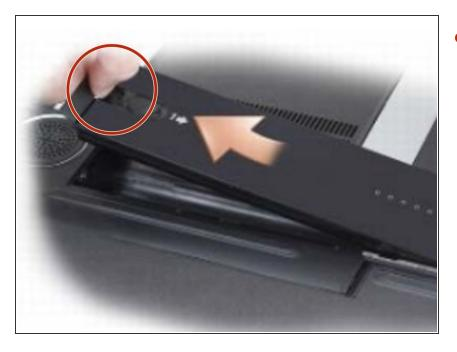
Lift the battery straight up and out of the computer.
