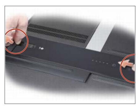
Using your thumbs, slide the battery in the direction of the #2 arrow by inserting one thumb into the recess
