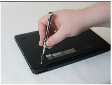
Remove the back 6mm and 8mm screws with a J000 screwdriver.
