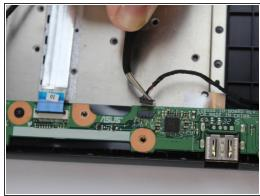
After unscrewing, gently unplug all the connections to the IO Board with tweezers. We have highlighted where these connections are located in our images.
