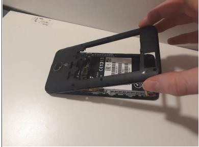
• Pry between the silver plastic layer and the screen. Go all around the device until it's seperated.
