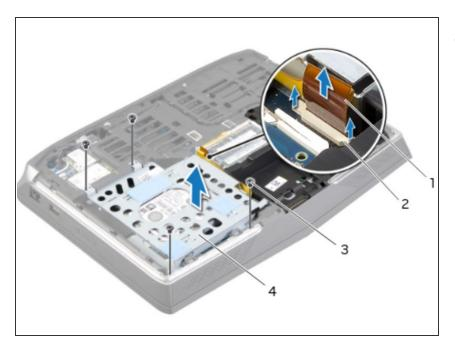
Turn the secondary hard-drive assembly over.
