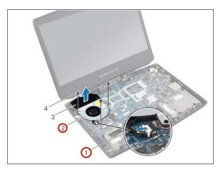
Lift the fan along with its cable away from the computer base.
