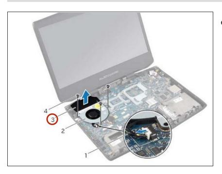
Route the camera cable on the fan and adhere the tape to the fan.
