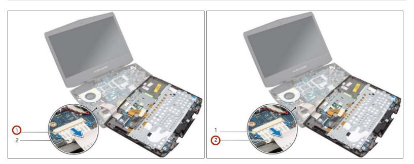
Release the connector latches to disconnect the flexi-cable from the system board.
