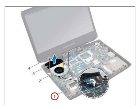
Disconnect the fan cable from the system-board connector.
