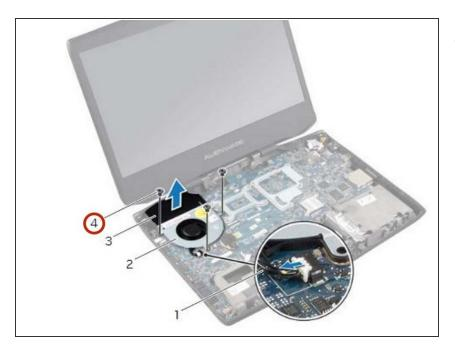
Remove the screws that secure the fan to the computer base.
