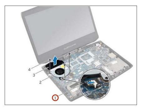
Connect **NEW** the fan cable to the system-board connector.
