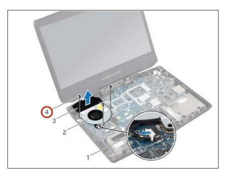
Align the screw holes on the fan with the screw holes on the computer base.
