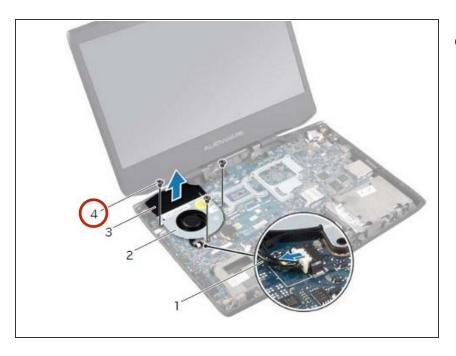
Replace the screws that secure the fan to the computer base.
