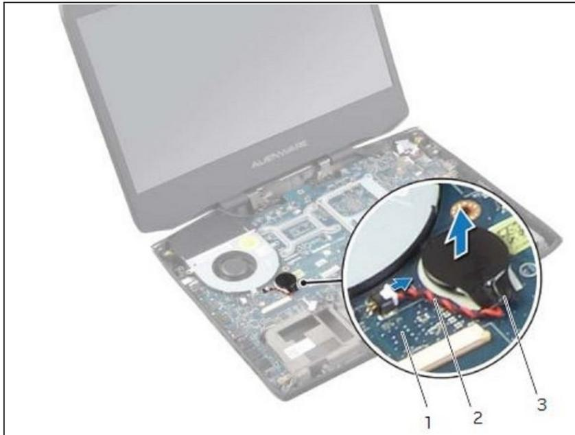
**⚠ WARNING:** The battery may explode if installed incorrectly. Replace the battery only with the same or equivalent type. Discard used batteries according to the manufacturer's instructions.
