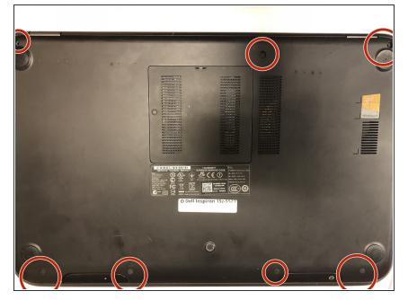
Remove all rubber stoppers and screw from the back of the laptop
