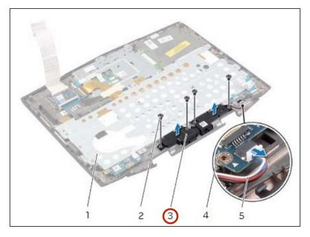
• Lift the speakers along with the its cable off the palm-rest assembly.
