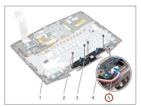
Route the speakers cable through the routing guide on the palm-rest assembly and connect the speakers
