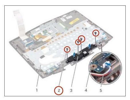
Align the screw holes on the NEW speakers with the screw holes on the palm-rest assembly.
