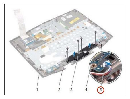
• Disconnect the speakers cable from the status-light board.
