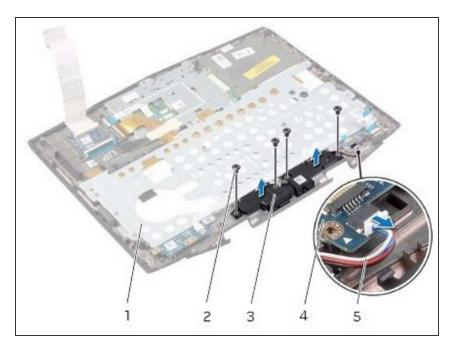
• Replace the screws that secure the speakers to the palm-rest assembly.
