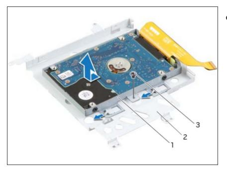
Turn the secondary hard-drive assembly over.
