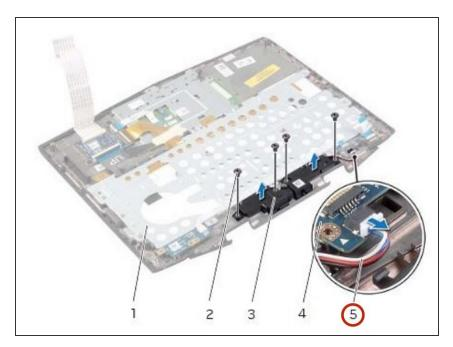
• Note the routing of the speakers cable and remove the cable from the routing guide.
