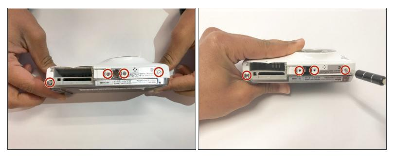
Remove all 4 screws from the bottom face of the camera using a Phillips #00 head screwdriver (found in iFixit tool kit).
