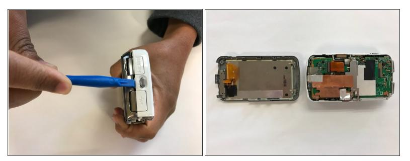
Using a plastic tool, pry open the back panel of the camera. Be careful not to apply too much force and damage the camera.
