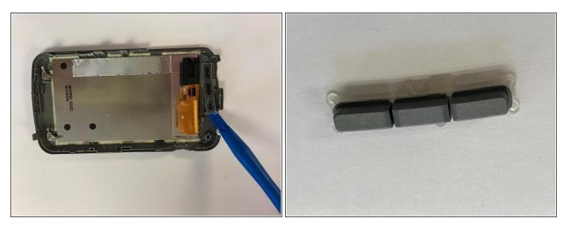
• Remove the selector button chain by prying it up with plastic tool of your choice.
