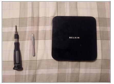
Pictured here is the Belkin F5L009, along with a plastic opening tool and a #1 Philips (at least so the head says...), which were the only tools I needed to do this. A guitar pick or other thin, flat, plastic object might work instead of an opening tool; I didn't test it.
