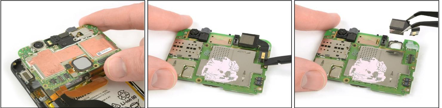
**⚠ The front facing camera and the headphone jack are still connected to the motherboard. Don't damage them while removing the motherboard.**
