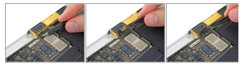
• Use tweezers to peel up the tape covering the two ZIF connectors—one for the right speaker cable, and one for the audio jack board cable.
