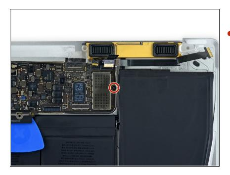
Remove the single 3.5 mm T5 Torx screw securing the logic board to the lower case.
