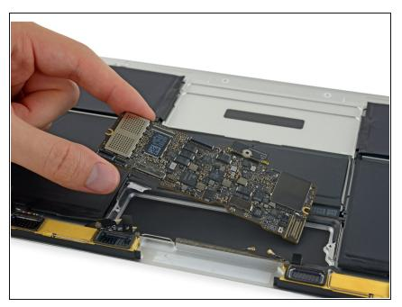
• Remove the logic board.
