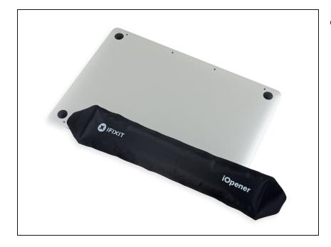
Prepare an iOpener and heat the lower case directly beneath the right speaker for 1-2 minutes, in order to soften up the adhesive securing the speaker.
