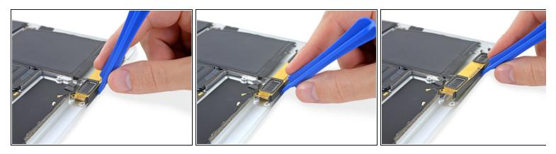
• Use a plastic opening tool to pry under the top edge of the left speaker, and separate it from the lower case.
