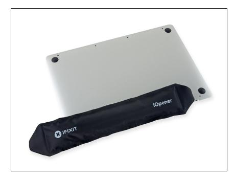
• <u>Prepare an iOpener</u> and heat the lower case directly beneath the left speaker, in order to soften up the adhesive securing the speaker.
