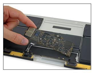
• Remove the logic board.
