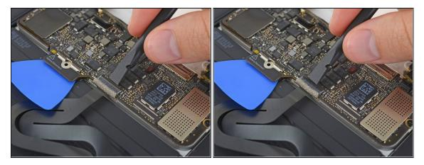
• Use a spudger to flip up the retaining flap on the trackpad cable ZIF connector.
