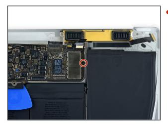
Remove the single 3.5 mm T5 Torx screw securing the logic board to the lower case.
