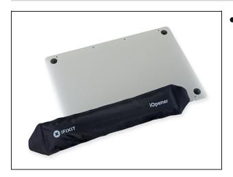
Prepare an iOpener and heat the lower case directly beneath the left speaker, in order to soften up the adhesive securing the speaker.
