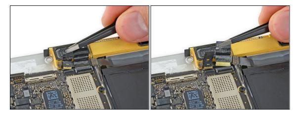
• Carefully pull straight back on the two pieces of tape you just peeled up to disconnect the two ribbon cables.
