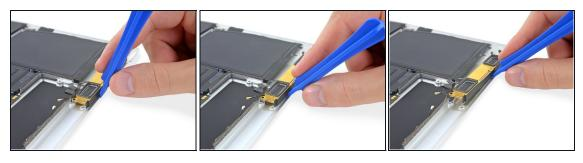
• Use a plastic opening tool to pry under the top edge of the left speaker, and separate it from the lower case.
