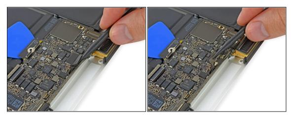
• Use the point of a spudger to peel up the foam pad covering the two antenna connectors.
