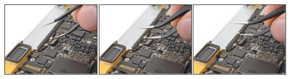
Insert one arm of your angled tweezers under the metal neck of the first antenna connector and pry up to disconnect it.
