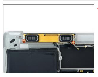
Remove the two 4.1 mm T3 Torx screws securing the left speaker to the lower case.
