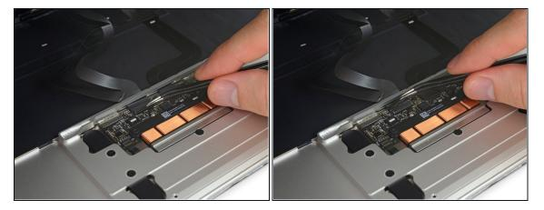
• Use tweezers to peel back the tape covering the trackpad cable ZIF connector.
