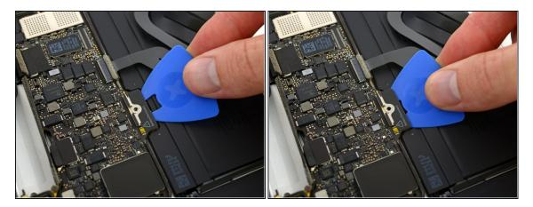
• As an added precaution, you may physically disconnect the battery by inserting a <u>battery isolation pick</u> between the logic board and the battery connector.
