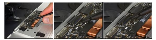
• Use a spudger to carefully flip up the retaining flap on the trackpad cable **ZIF** connector.
